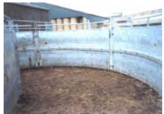
Figure 3: A curved forcing pen with holes for a spring loaded pin to prevent accidental movement of the forcing gate.
